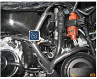
To disconnect the rail pressure plug press the locking lever. Connect the rail pressure adapter in between both connections.
