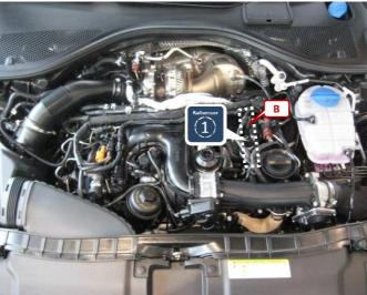
Localise the common rail bar (B). The rail pressure sensor is located in the middle from the common rail bar.
