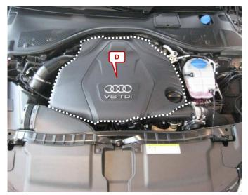
Open the engine hood. Remove the engine cover (D). The engine cover is not screwed.
