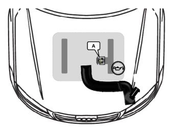
A Rail pressure sensor (3 pin)
