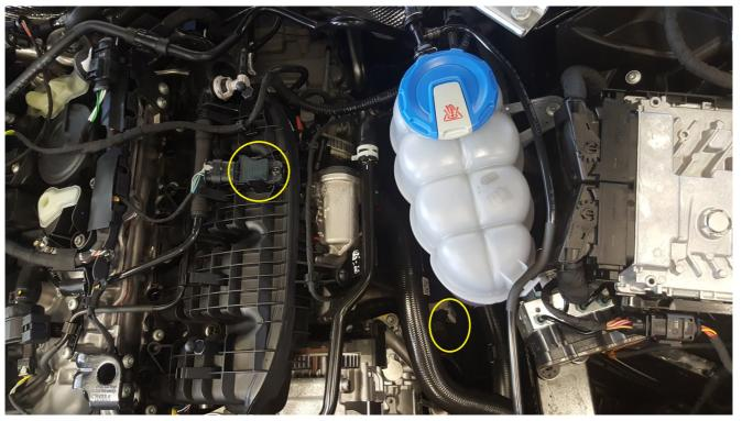
Localise the top front area of the engine compartment. The 4-pin intake manifold pressure sensor is located centered in this area.
