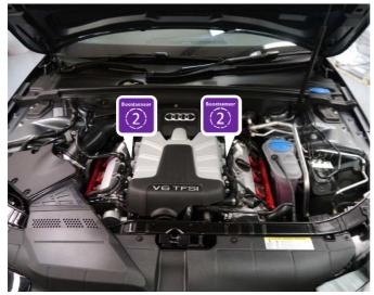
Open the engine hood. Localise the intake manifold sensors on each side from the engine.
