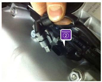
Press the locking lever to disconnect the sensor
