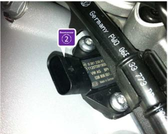
Connect the adapter cable with both sensors. Connect then the original sensor plug with the adapter cable. Move the adapter cable not in parallel with injection pipelines ABS-control device connecting leads. Keep to very big distances. Fix the adapter cable with cable ties. Connect the module to the adapter cable. Check all connections and reassemble the vehicle in reverse again order.
