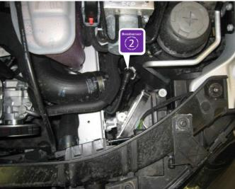
The 4-pin boost pressure sensor is right at the pressure pipe behind the headlight.
