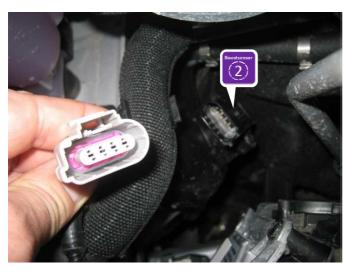
Open the plug by pulling the locking lever and connect the boost pressure adapter in between both connections.
