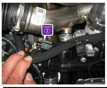
Localise the left front area from the engine compartment. The 4-pin boost pressure sensor is located at the pressure pipe before the throttle bodys.
