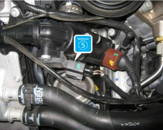
Localise the front, right area from the engine compartment. The boost pressure sensor is located in the front right area from the engine at the pressure pipe before the throttle bodys.
