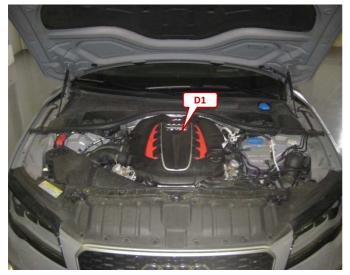
Open the engine hood. Remove the engine cover (D1). The cover is not screwed.
