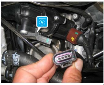
Open the plug by pulling the locking lever and connect the boost pressure adapter in between both connections.
