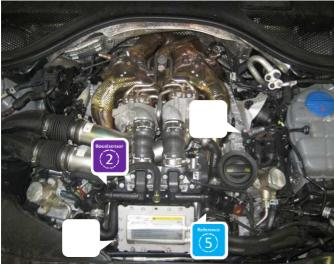
Connect the system to these two boost pressure sensors . The boost pressure sensors are located in the front left and right area from the engine at the pressure pipe before the throttle bodys. Number 2 and 5
