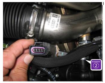
connect the boost pressure adapter in between both connections.
